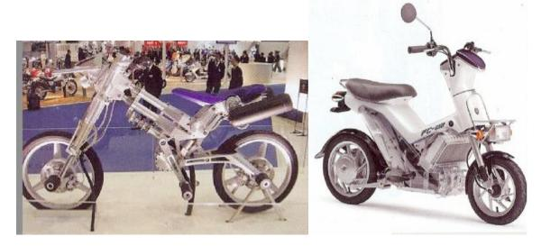
The FC-me from Yamaha, shown above right is a production fuel cell powered scooter. It is powered by a methanol fuel cell producing electricity to drive an electric motor. The alcohol will not freeze at reasonably cold temperatures. These are currently available for lease by city governments. Units similar to this have already passed durability testing which included real life driving in city traffic.
