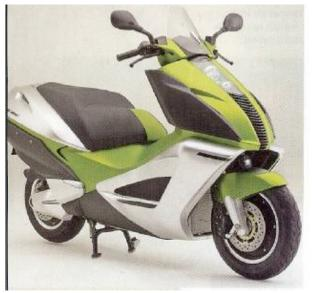
Yamaha's HV-1 is a hybrid scooter concept shown above left. It is powered by both electric and gasoline motors. The scooter can be driven in a quiet mode on electric only. The electric motor can also be used to help park the bike in tight situations. The gasoline motor extends the cruising range of the bike.
