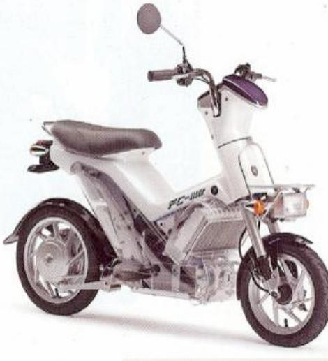
The FC-me from Yamaha, shown above right is a production fuel cell powered scooter. It is powered by a methanol fuel cell producing electricity to drive an electric motor. The alcohol will not freeze at reasonably cold temperatures. These are currently available for lease by city governments. Units similar to this have already passed durability testing which included real life driving in city traffic.
