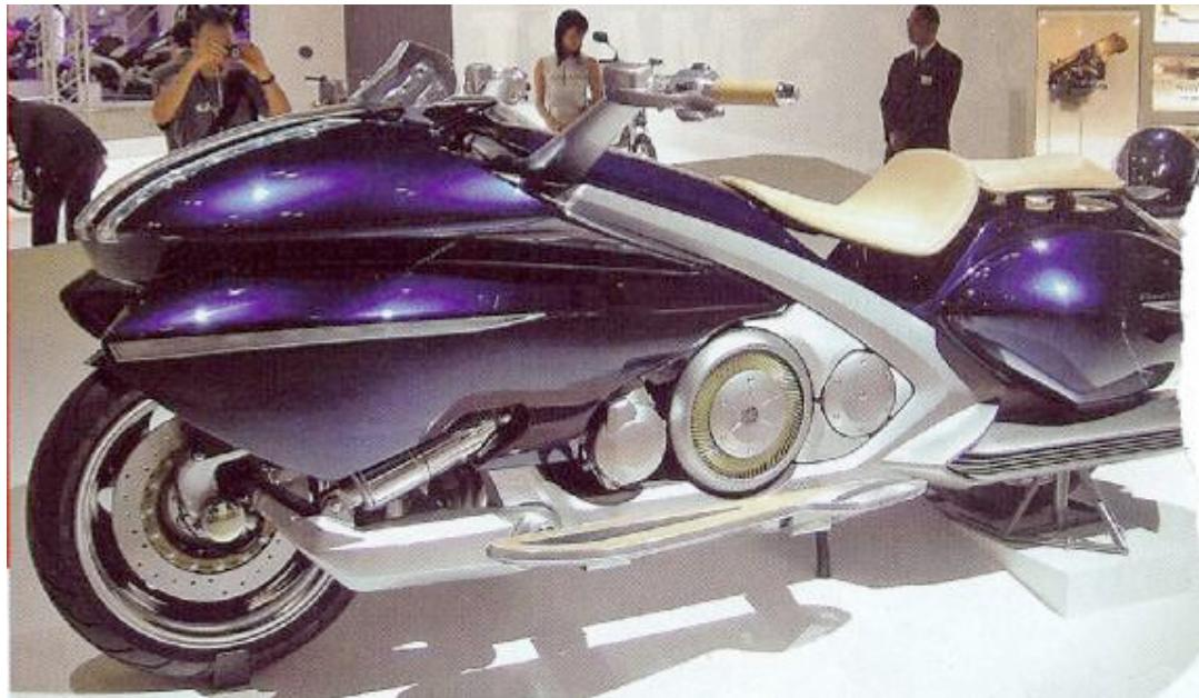
Yamaha's concept for midsize/full size hybrid motorcycle is shown above. It has a 600cm<sup>3</sup> gas engine coupled with an electric motor. The electric motor can be used simultaneously with the gas motor to provide higher performance.
